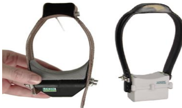
Figure 7. GPS collars: (Left) , GPS collar designed for small mammals, (Right) GPS collar designed from medium-large sized mammals (Images provided by Lotek Wireless Inc. [118]).
