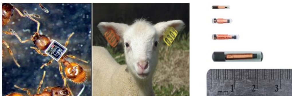
Figure 6. (Left) A radio tagged ant (Reproduced with permission from RFID Journal, 1 August 2009. Image, and copyright held, by, Nigel R. Franks) [107], (Middle) Passive RFID ear tags (Image provided by Premier1Supplies [108]), (Right) Passive RFID implants (Image provided by Biomark Inc. [109]).
