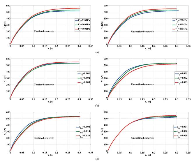
Fig. 4 Influence of the concrete parameters of the structure on the Pushover curve; (a) concrete compressive stress, (b) peak strain corresponding to concrete compressive strength  $\varepsilon_{c0}$  and (c) ultimate deformation of concrete
