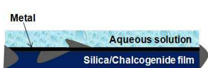
Figure 1. Schematic configuration for three layer SMA sensor.
