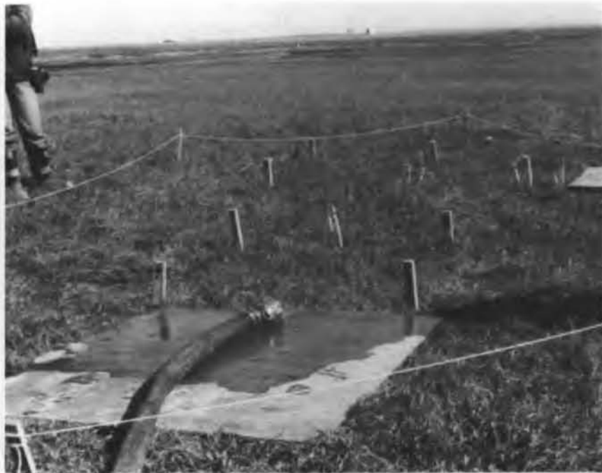
Figure 3. Application of seawater at the West Dock mesic site. The plastic tubes attached to the lysimeters can be seen at the center and the right.
