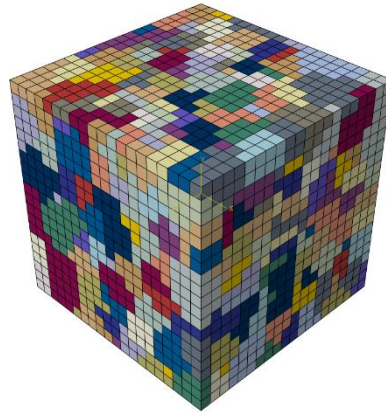
Figure 1. Summary of the mesh used in the simulations, consisting of approximately 700 grains with a 14 \mu\text{m} mean grain diameter. Element size is 5 \mu\text{m} and side lengths of the cube are 100 \mu\text{m} .
