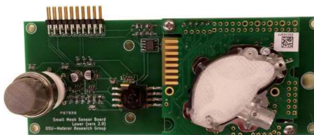
Fig. 12 A picture of the sensor board with encapsulating materials removed.
