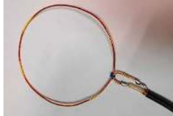
Fig. 5. Single loop antenna (antenna diameter 95 mm, wire diameter 1.2 mm, bandwidth 20 MHz corresponding to 2:1 VSWR, voltage standing wave ratio, using a 50 Ohm termination at the oscilloscope input) used for radio frequency corona detection.
