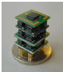
Fig. 1 The four layers of the IMEC Sensor Cube hardware platform. A 2€ coin provides a size reference.
