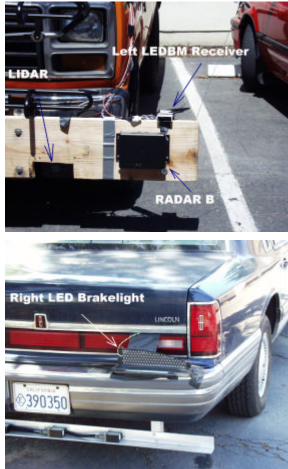
Figure 3. Mounting of LEDBM System and Test Components
