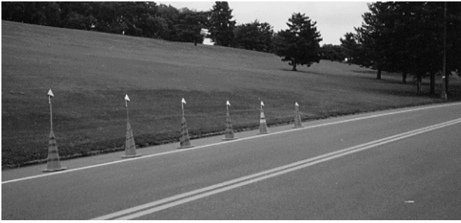
Fig. 2. Roadside-deployed basic {111111} array of radar-reflecting corner cubes
