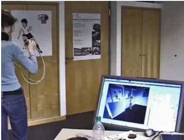
Figure 6.10: The sensor unit is tracked in a large room. The monitor shows the live camera image augmented with a virtual character.
