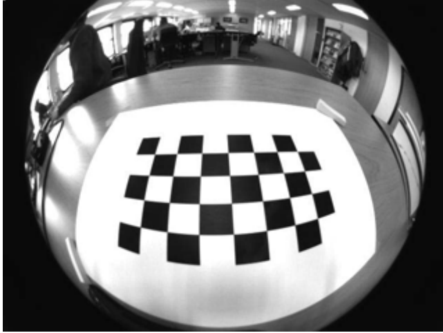
Figure 3.11: A typical image used for camera calibration. The calibration object is a planar checkerboard pattern with known dimensions.
