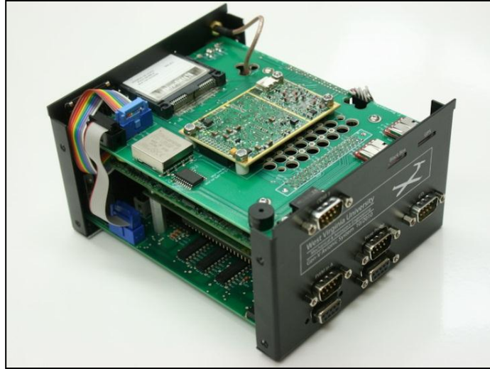
Figure 3.5: Gen-V avionics system in custom enclosure.
