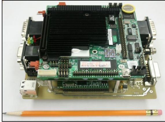
Figure 3.4: Bottom three stacks of Gen-V avionics system [72].
