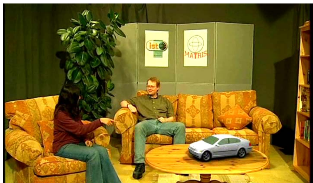
Figure 1: An example of how AR can be used in TV production: a virtual car has been rendered into the scene.
