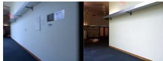
(b) Appearance proposal with a high scan-matching score - correctly rejected as only a single line feature is present.
