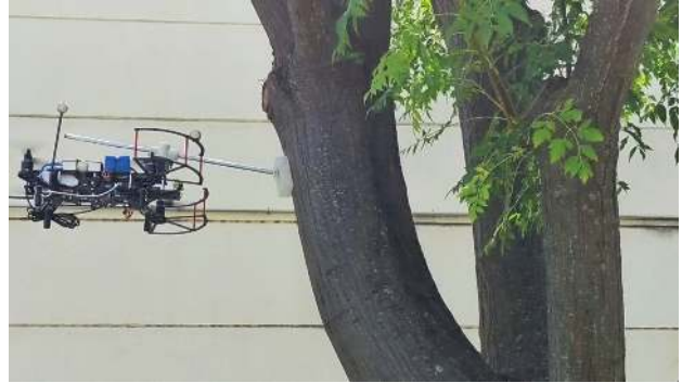
Fig. 1: A small-sized quadcopter equipped with the bespoke lightweight manipulator performs installation of a sensor on a tree.
