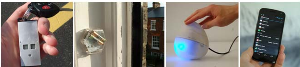
Figure 9. IOT Home Automation and Environment Monitoring Innovations: Sensordrone, Flexibility Internet Sensors, Air Quality Egg, and openHAB on Android.
