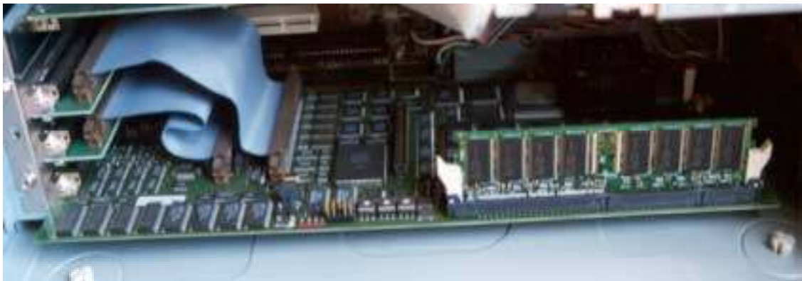
Fig. A.6.3 DS1103 inside the Pentium PC
