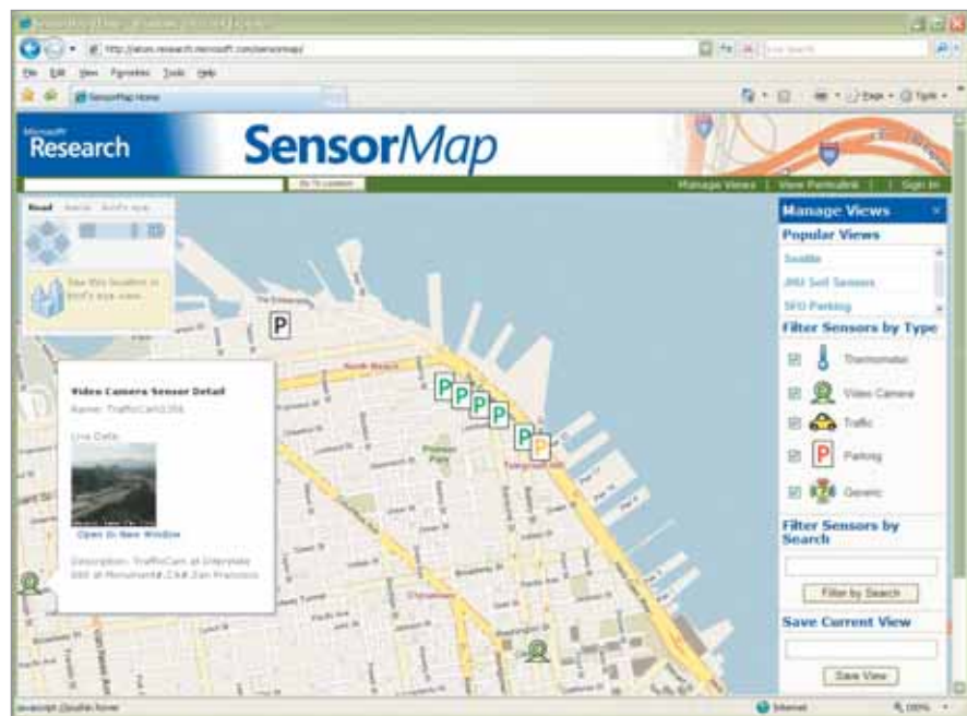
Figure 2. SensorMap GUI. Based on Windows Live Local, the GUI provides zooming, panning, street maps, satellite images, and 3D views.
