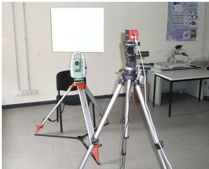
Figure 8. System used to evaluate the influence of the alpha angle on camera distance measurements.
