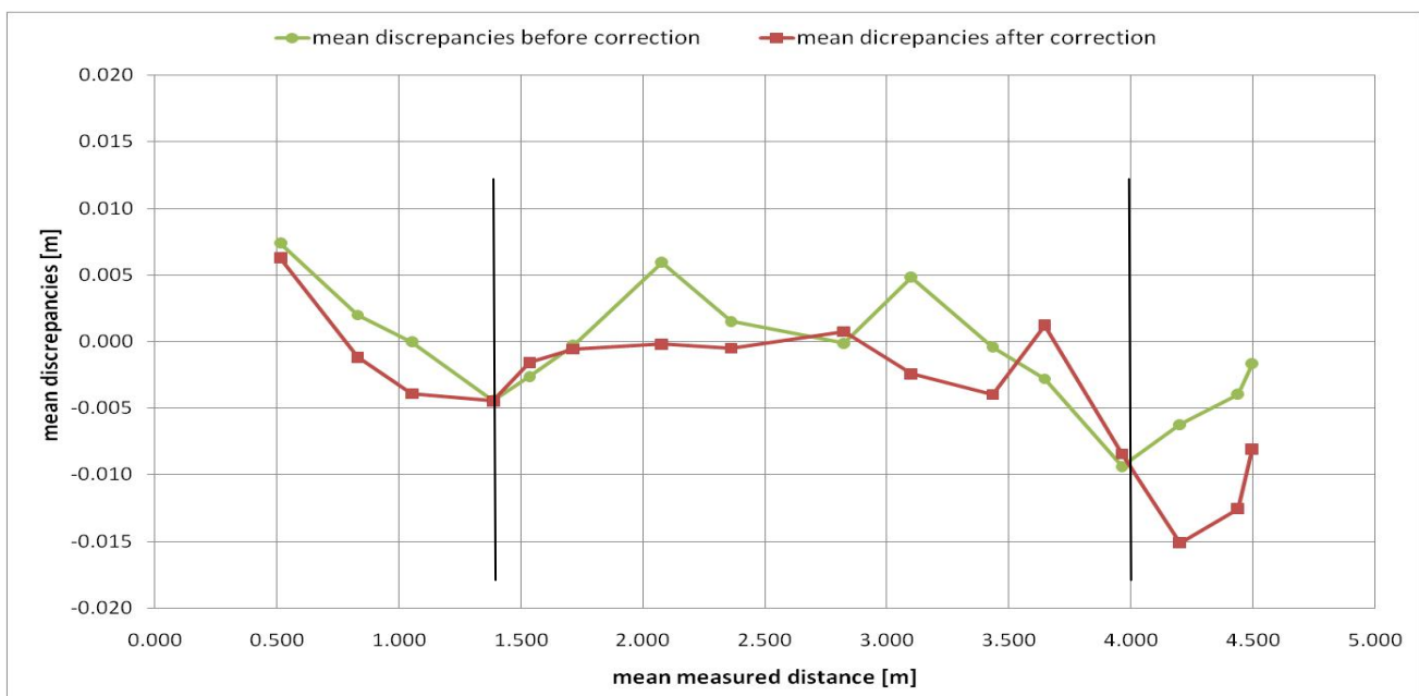
Figure 6. Mean values of the discrepancies ( g ) of all the considered pixels before and after distance error model correction.
