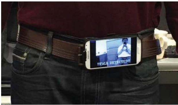
FIGURE 7. An Android smartphone attached to the waist.
