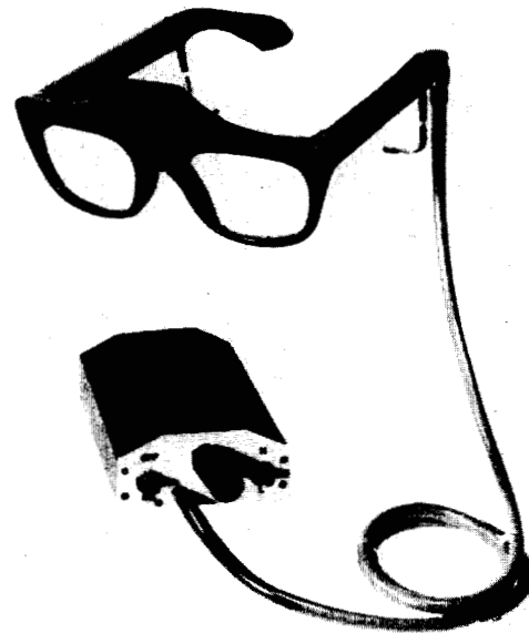
Fig. 12. The Ultrasonic Spectacles designed by Kay. Transmitters and receivers are located at the bridge of the nose. Batteries are located in a vest pocket carrying case.
