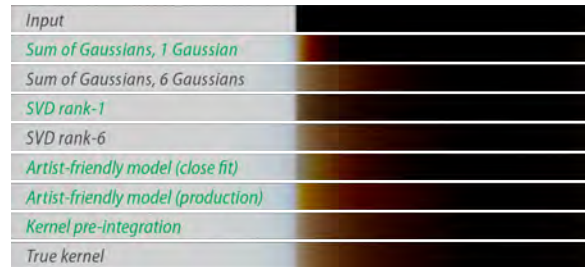
Figure 7: Comparison of the results for our two separable techniques applied to a step-like irradiance: both the sum-of-Gaussians [dLE07, JSG09] and a low-rank SVD-based decomposition need several convolutions to match the true kernel. Our proposed pre-integrated kernel, however, is exact for axis-aligned functions, such as this example. Our artist-friendly model provides a rich design space: This is illustrated by two approximations, where for the first (close fit), perceptual similarity to the ground truth was the modeling objective, while the second (production) was tweaked by an artist for production purposes. Note that the image is best viewed in the electronic version of the paper. The style of presentation was inspired by previous work [DI11, HCJ13]. Additional 2D visualizations of the different kernels are provided in the supplementary materials, where we also demonstrate that the radial asymmetry of the SVD-based kernels vanishes rapidly with increasing rank.
