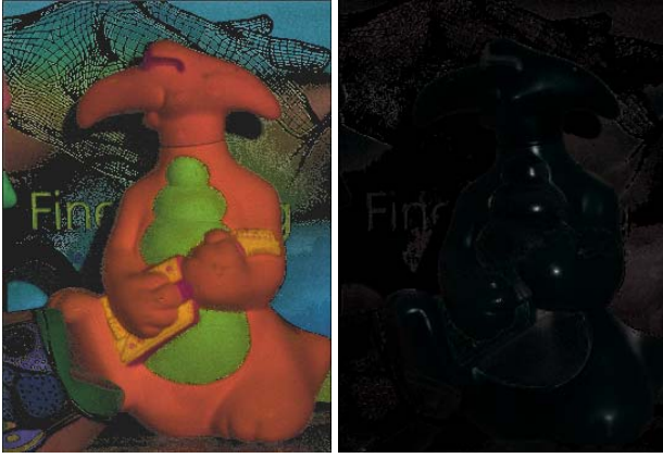
Figure 5: a. Diffuse component of Figure 3.a b. Specular component of Figure 3.a
