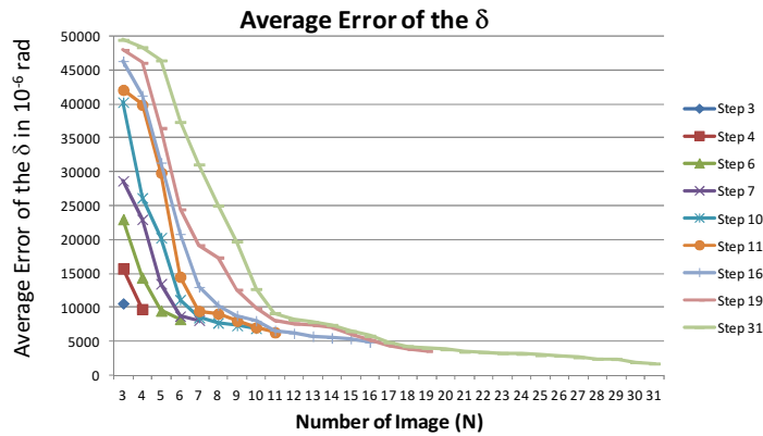
Fig. 6. A plot of the average error in 10^{-6} rad versus the number of frames ( N ) for angle \delta .
