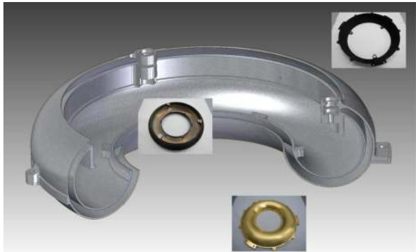
Fig. 34 Electrostatic Analyser (ESA), consisting of three parts, which are screwed together
