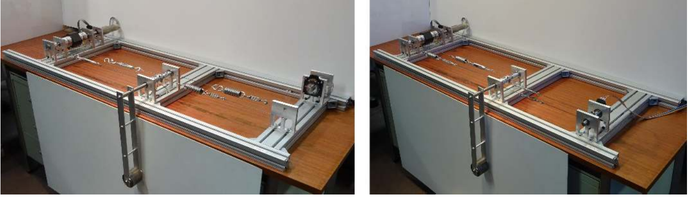
Fig. 5: Experimental setup: PEA (left) and SEA (right) configuration. Gearbox and output shaft are equipped with incremental encoders. Additionally, a torque sensor is included at the gearbox output. The length of the drive train, output shaft, and pendulum are 0.44[m] , 0.27[m] , and 0.40[m] , respectively.
