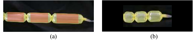
Fig. 5. (a) sPAM with o-ring spacing too large. Regions highlighted in red are where pleated PAM model predicts bulge radius larger than D_{\text{tube}} , and hence they do not contribute to contraction. (b) sPAM without inactive regions.
