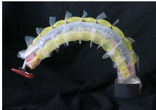
Fig. 1. Soft continuum robot with series pneumatic artificial muscles (sPAMs) attached.
