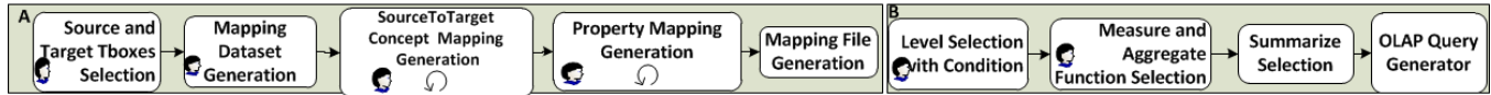
Figure 2: The workflows for Source2Target Mapping(A) and OLAP Query Generation (B) operation. The rectangles, user icons and curved arrows represent automatic, user-required and iterative tasks.
