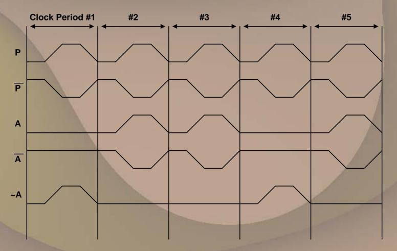
A = voltage inverse of A, ~A=logical inverse of A
