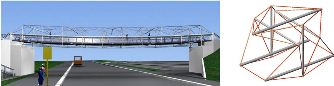
Fig. 11 The 2003 TorVergata Footbridge project and one of its TS modules, as redesigned in 2006
