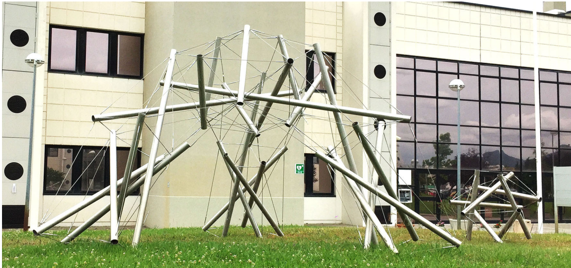
Fig. 18 A three-legged structure and a seven-bar module designed with the procedure presented in [88] (photo courtesy of Paolo Cignoni, CNR-ISTI)
