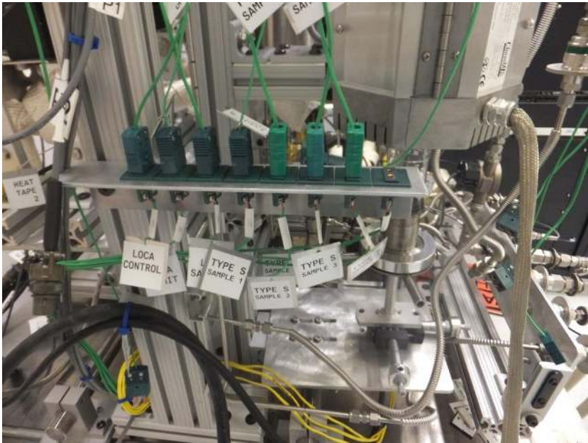
Figure 37 Thermocouple panel of the in-cell LOCA system.
