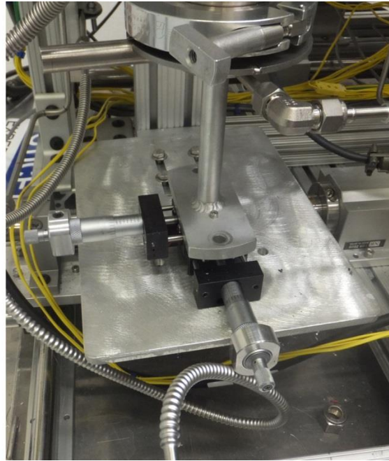
Figure 34 Furnace bases of the out-of-cell (left) and in-cell (right) attachments for the LOCA furnaces.
