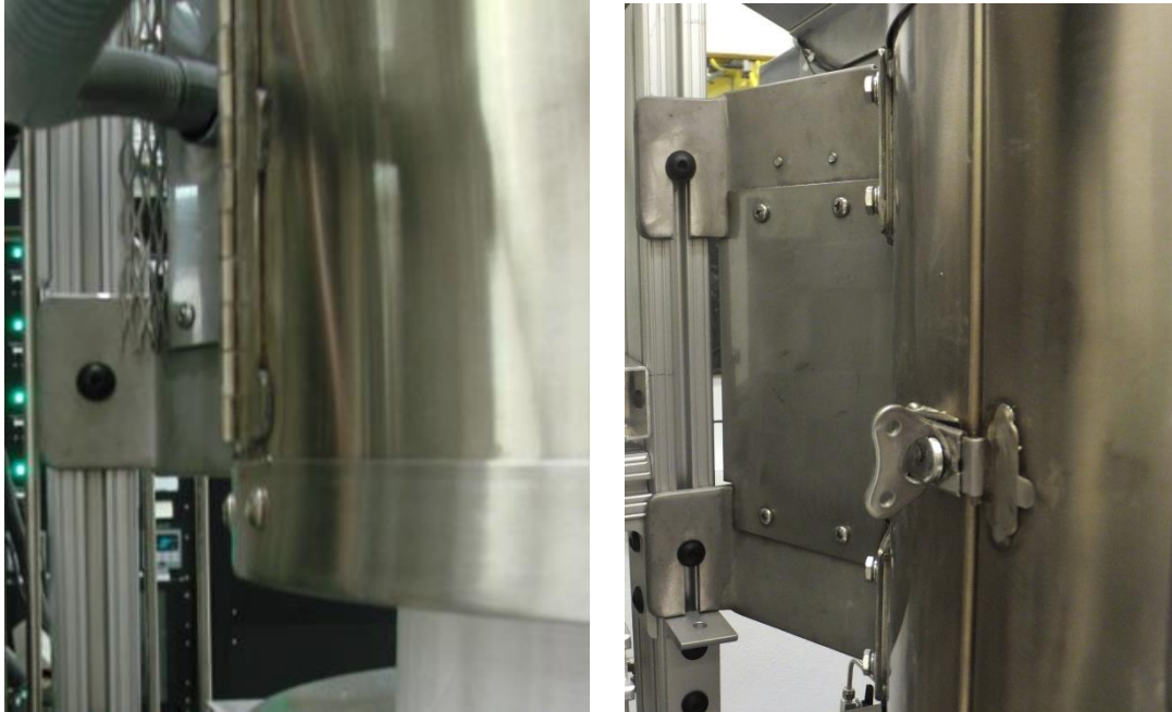
Figure 28 Furnace bracket arrangements on the out-of-cell (left) and in-cell (right) attachments for the high temperature furnaces
