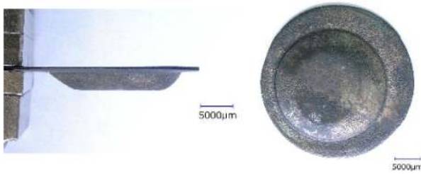
Fig. 23 Appearance of Inconel 718 sheet sample after 8 passes of IF-HPS processing, and extracted circular area surrounded by dotted line (upper). Side and top views after cup-forming of extracted circular disk (lower). 160)
