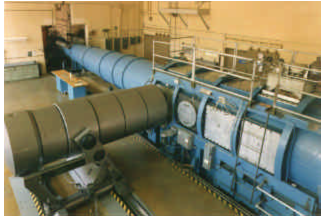
Figure 12 – AEDC White Oak Tunnel 9 facilities. The wind tunnel can be configured for a variety of different flow conditions and Mach numbers.
