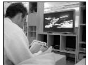
Figure 6.5: The current version of LOCOMOTION consists of two tablet computers and a PC with a plasma screen connected over the network.
