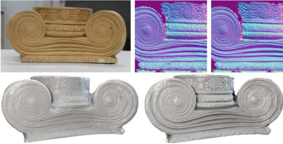
Fig. 8. The Figure dataset. Top from left to right: An input image of the dataset; normal maps from the surface computed by our implementation of Semerjian [5], and our shading based approach. Bottom: Result presented by Zollhoefer et al. [3] (available at project website); and our fused model.
