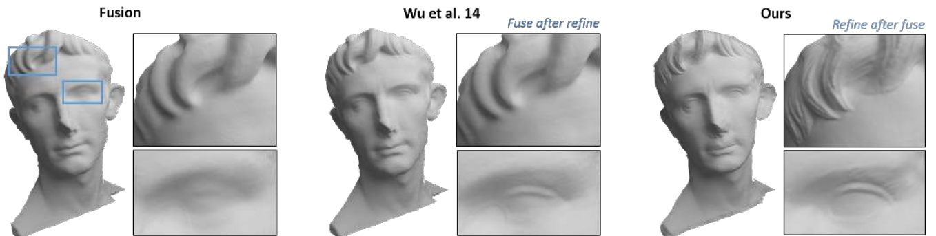
Figure 13: The method of Wu et al. [2014] refines independent depth maps, causing detail to smooth out in the subsequent fusion process; i.e., fuse after refine. Our method refines the geometry after surface fusion, i.e., refine after fuse, thus capturing substantially more detail.
