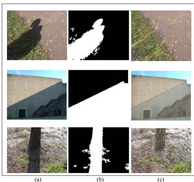
Fig. 5. Results of the shadow detection and removal algorithm: original images containing a shadow (a); shadows detected shown in white (b); output of the proposed method (c)
