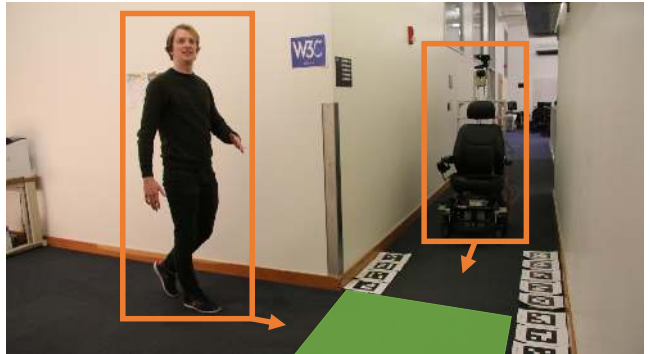
Fig. 1: The proposed ShadowCam algorithm detects moving obstacles behind a corner which cast a shadow in the marked green area. This makes driving with the autonomous wheelchair safer by avoiding dangerous potential collision situations.
