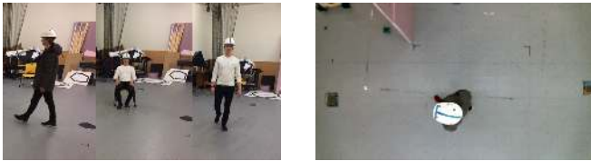
Fig. 6: The left image shows how we varied the size of the moving object behind the corner: Wearing a winter jacket, sitting on a chair with rollers and walking normally. The right image shows the corner wall and a person walking from the top view.
