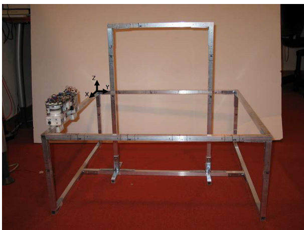
Fig. 5. This figure shows the Shady3D testing environment. The origin is the left-rear corner of the horizontal frame in the image (marked by the XYZ frame). Indices and gripper boundaries are marked for the nodes. The vertical frame in the middle is located so that an individual Shady3D robot can move from the surrounding horizontal frame to the vertical frame by itself.
