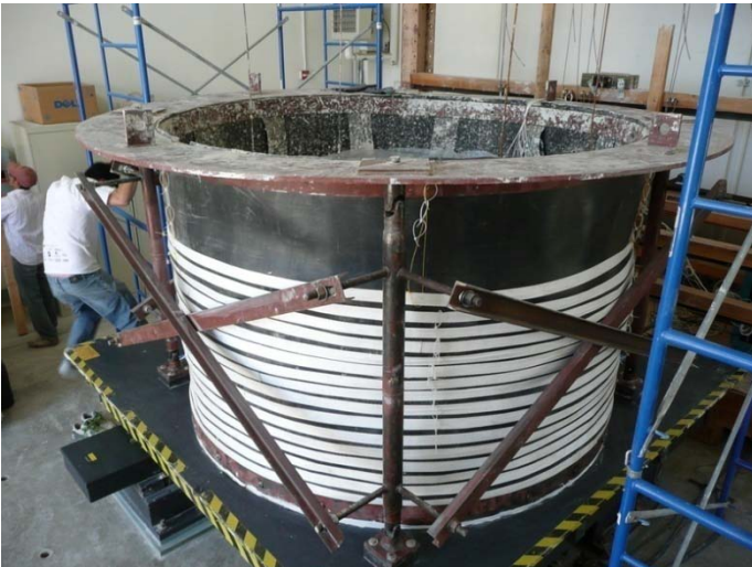
Figure 5. Shown is a full barrel being prepared for initial calibration tests. Note the cross bracing still in place that will be removed prior to testing to allow the flexible wall barrel free movement in response to the imposed shaking.
