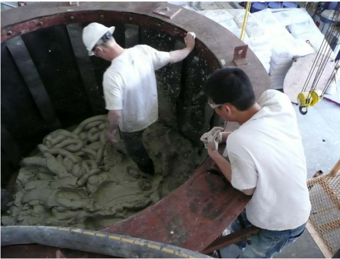
Figure 4. Process of filling the barrel with scale model soil. Ten accelerometers were placed in the soil lifts in both vertical and horizontal arrays to record the dynamic response of the soil during shaking.
