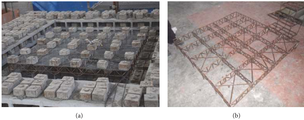
FIGURE 8: Overview and structural components of “Treasures fill the house”: (a) specimen; (b) joints.
