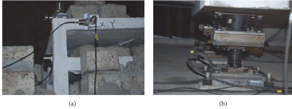
FIGURE 10: Arrangement diagram of sensors: (a) acceleration sensors; (b) three-directional force sensors.
