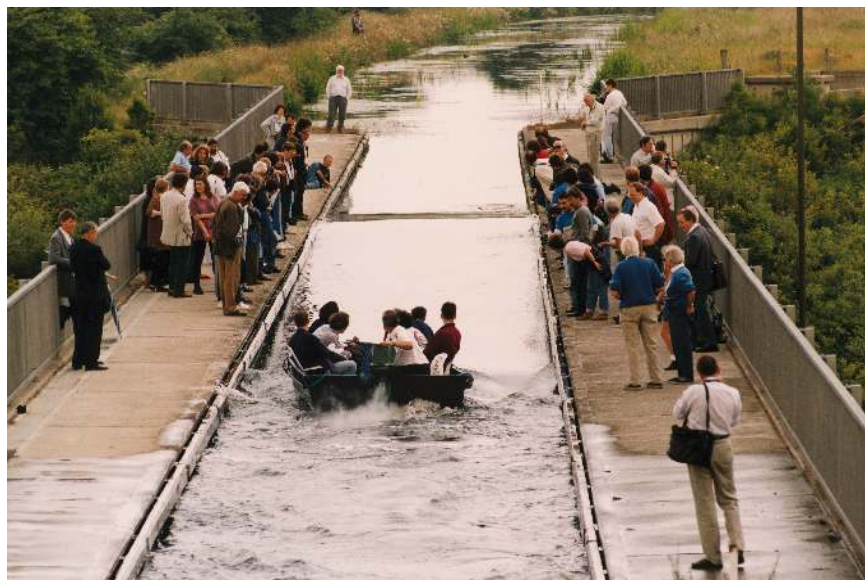
Figure 3: Recreation of a solitary wave on the Scott Russell Aqueduct on the Union Canal. Photograph courtesy of Heriot-Watt University.
