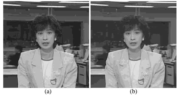
Figure 12. Reconstructed Announcer images in which region-of-interest is encoded with increased quality and background area is encoded with reduced quality: (a) SA-DCT, (b) SA-APIDCBT.
