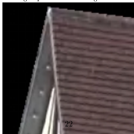
(c) 2x enlarged portion of the reconstructed visual object at 0.8889bpp using SA-DWT coding in MPEG-4 (PSNR-Y=32.73dB; PSNR-U=42.26dB; PSNR-V=42.43dB).
