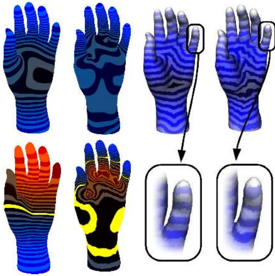
Figure 4: Different functions calculated on the human hand. The first two top represent ADF for t=1 and t=0.1 , the bottom two are the Fiedler vector and highly smoothed Gaussian curvature, and the last two are geodesic based (pure geodesic and enhanced by the curvature) from [Tie08] (pictures used with the author's permission).
