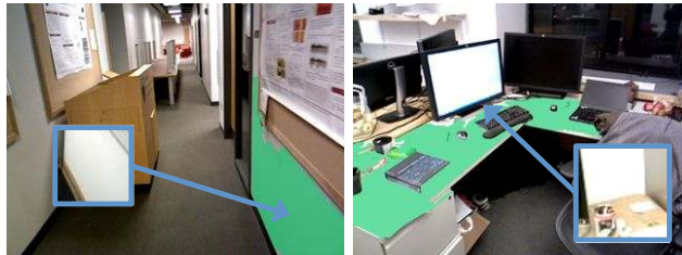
Figure 5. Plane extrapolation. If a shape anchor’s reconstruction is mostly planar, we infer the support of the plane (green). We also show the database matches for the two shape anchors.
