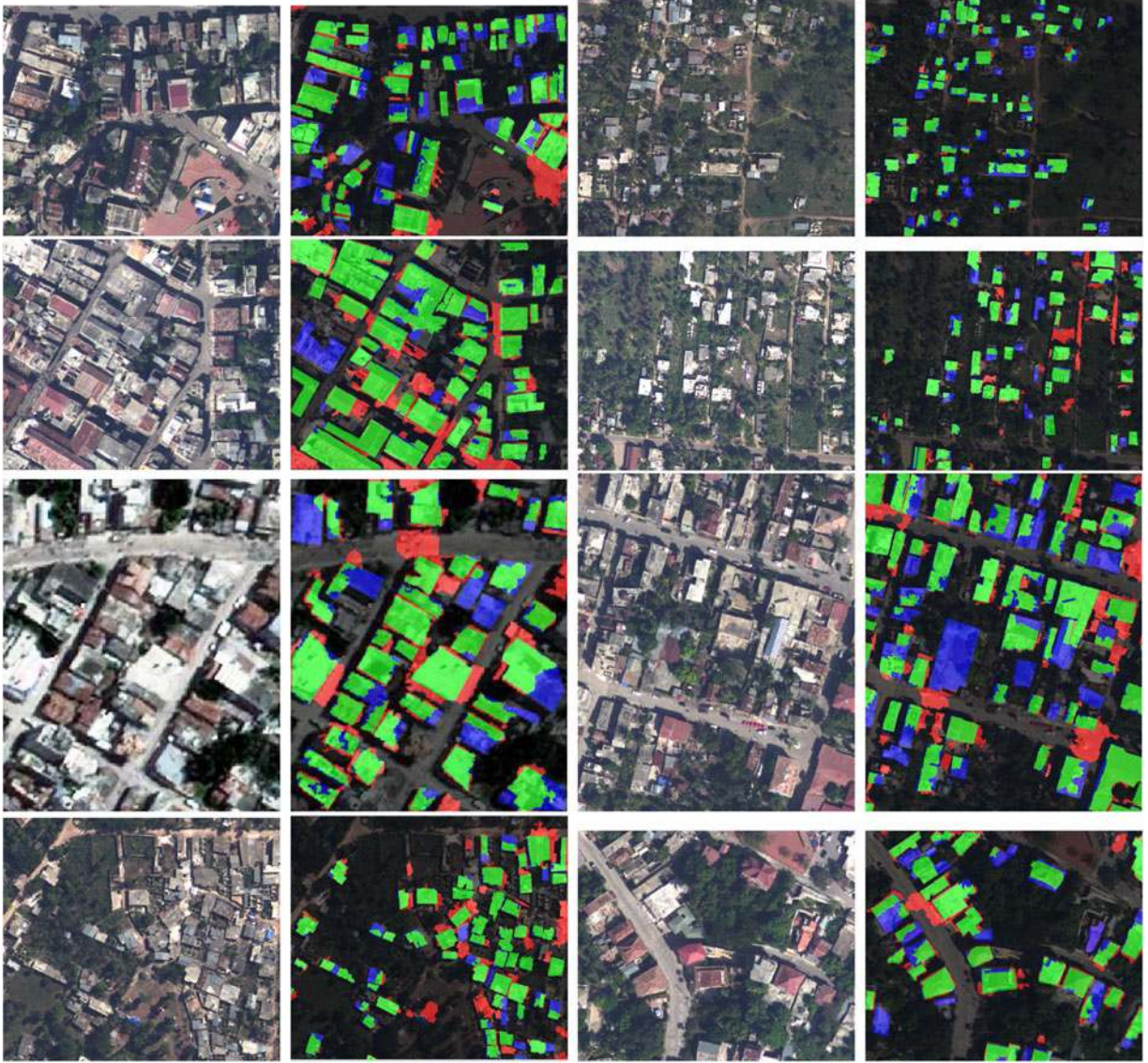
Fig. 8. The results of the proposed approach on NOAA images: (First column) Test images #1–4. (Second column) Detected buildings for test images #1–4. (Third column) Test images #5–8. (Fourth column) Detected buildings for test images #5–8.
