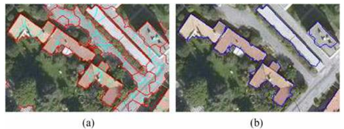
Fig. 7. Determination of final buildings: Three buildings (left) are approximated by the recursive MBR of level 2 and other two buildings (right) are rectangular. Their RMBR scores are, respectively, 0.87, 0.91, 0.84, 0.93, 0.81 (from left to right). The value of T_B is chosen as 0.8. (a) Segmentation result. (b) Final building.
