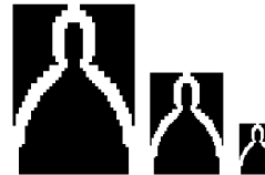
Figure 8: Binary model used to localize the pedestrian's head: different sizes are considered.
