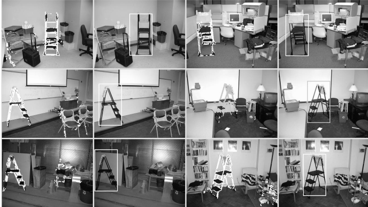
Figure 4. Results of edge filtering and edge grouping for cascades trained on various environments. For each pair of images, the left-hand image shows results of the edge filtering operation described in Section 2, and the right-hand image shows results of edge grouping as described in 3.3. Top row: The lab (left) and cubicle (right). Middle row: The classroom (left) and conference room (right). Bottom row: the warehouse (left) and living room (right).
