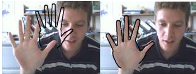
Figure 4: Hand localization and model alignment. The images show the initialization phase of a model-based tracker. The hand is located using chamfer matching and subsequently aligned by optimization. The right image shows the projected contours of the adapted model,
